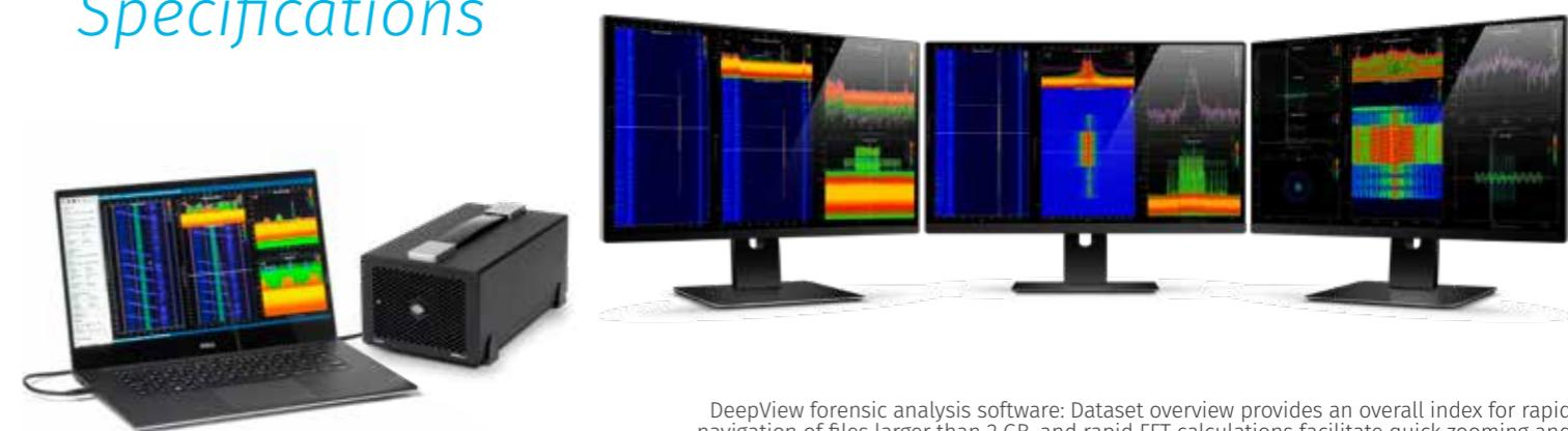
DeepView forensic analysis software: Dataset overview provides an overall index for rapid navigation of files larger than 2 GB, and rapid FFT calculations facilitate quick zooming and reduced lag. Includes statistically weighted displays for frequency, time, power and I/Q along with many other powerful real-time and historical data analysis options.
